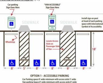
4. At least 1 per25 spaces is clearly marked with access symbol on vertical signs and on pavement. (S)
